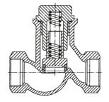
Fig. 4 RJ205Z Check valve
