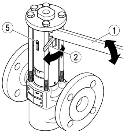
The pressed lever is under spring force.
