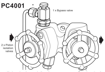
\* Please note that the line drain outlet is shown out of position for clarity and that the line drain pipework is to be supplied by the customer.
