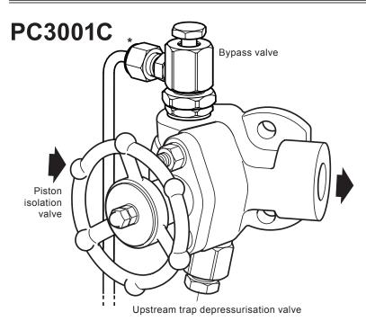
\* Please note that the line drain outlet is shown out of position for clarity and that the line drain pipework is to be supplied by the customer.
