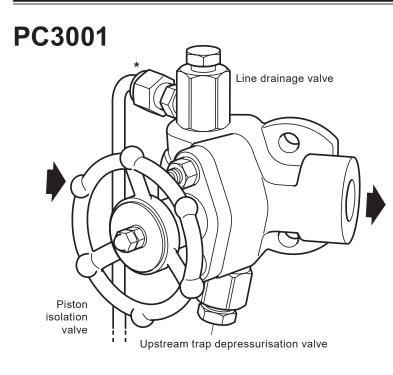
\* **Please note** that the line drain outlet is shown out of position for clarity and that the line drain pipework is to be supplied by the customer.
