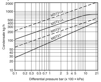
Cold water capacity - - - - Hot water capacity -
