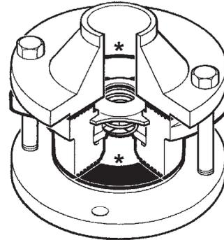
\* **Note:** Flanges, bolts (or studs), nuts and joint gaskets are to be provided by the installer. Disc check valves are non-maintainable (no spares are available). Disc check valves are not suitable for use where heavily pulsating flow exists, such as close to a compressor.
