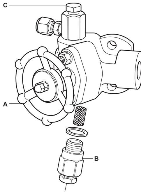
**Please note** when isolating the unit for strainer screen replacement drain any residue pressure through opening valve (B) **DO NOT break open the upstream drain until it has been drained.**
