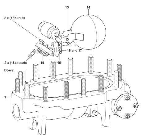
Fig. 7 Mechansim assembly removal
