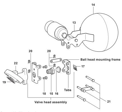
Fig. 9 Seat and ball head replacement
