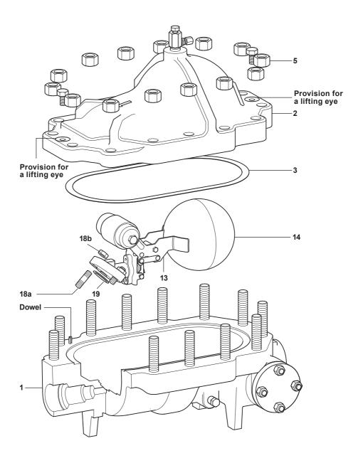
Fig. 10 Replacement fixed and mechanism assembly
