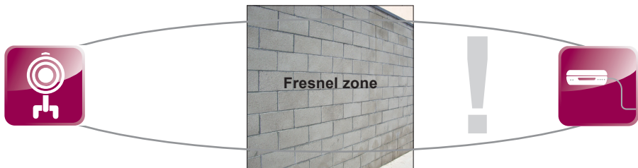
Fig. 5 Fresnel zone with blockage (obstacle) - Bad
