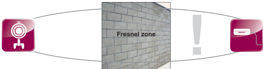
Fig. 6 Fresnel zone with blockage (obstacle) - Bad
