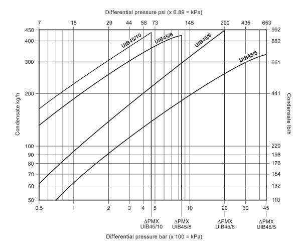
**Note:** Trap should be selected for the most appropriate working pressure differential and not on the basis of load. e.g. 80 kg/h at 7 bar (176 lb/h at 102 psi) differential should be handled with the UIB45/8 and not the UIB45/5.
