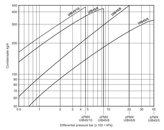
**Note:** Trap should be selected for the most appropriate working pressure differential and not on the basis of load. e.g. 80 kg/h at 7 bar differential should be handled with the UIB45/8 and not the UIB45/5.
