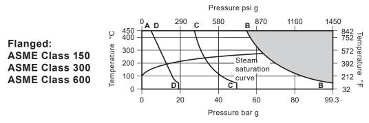
The product must not be used in this region or beyond the parameter of the PMA or TMA of the relative end connection.
