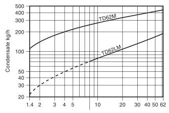
Minimum operating pressure 8 bar for the TD62LM Differential pressure bar (x 100 = kPa)
