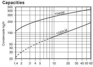
Minimum operating pressure 8 bar for the TD62LM
