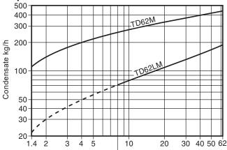
Minimum operating pressure 8 bar for the TD62LM
