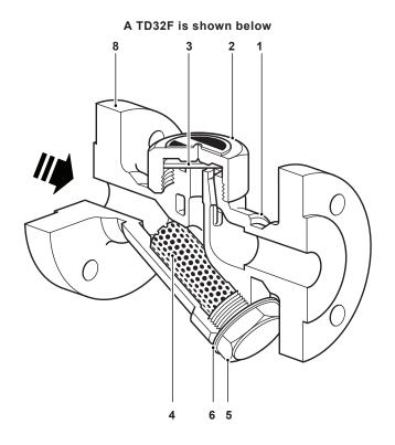
The TD32FALC version is identified by the groove in the cap
