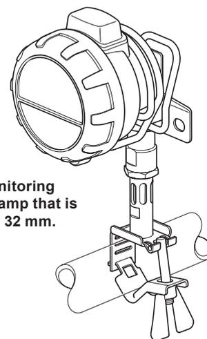
Wireless steam trap monitoring system plus jubilee clamp that is used on pipelines from 40 mm to 100 mm.
