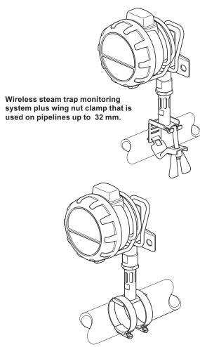
Wireless steam trap monitoring system plus jubilee clamp that is used on pipelines from 40 mm to 100 mm.
