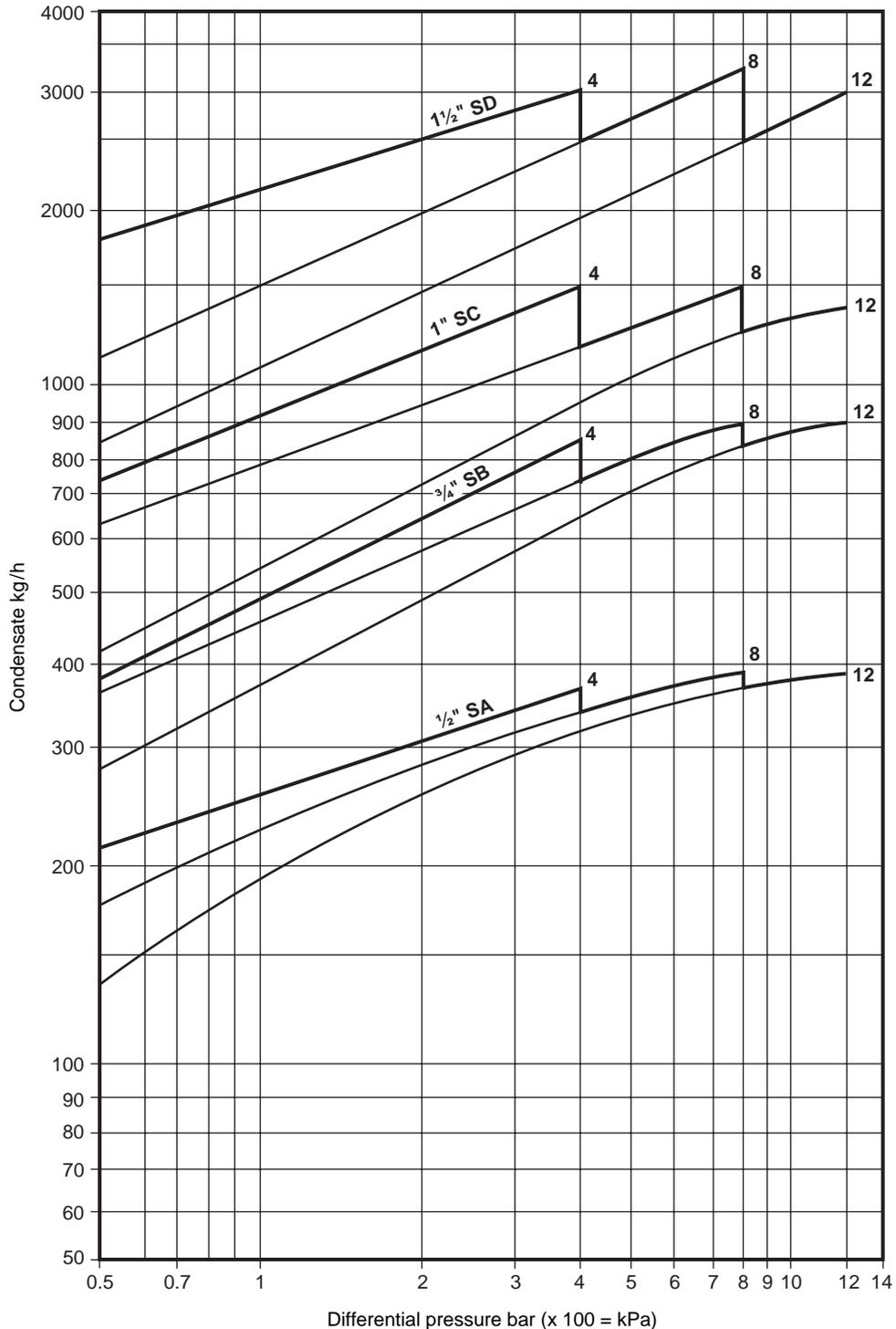
**Note:** Traps should be selected for the most appropriate working pressure differential and not on the basis of load.
