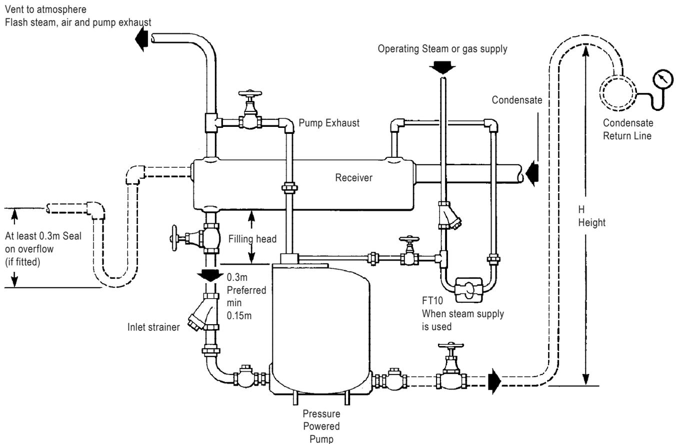
Recommended installation of pressure powered pump when fitted to a vented receiver. Flash steam must be vented or condensed ahead of pump inlet. Application details will dictate which of the following options will be necessary to accomplish this.
