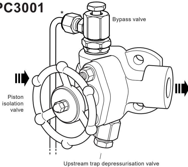
\* **Please note** that the line drain outlet is shown out of position for clarity and that the line drain pipework is to be supplied by the customer.
