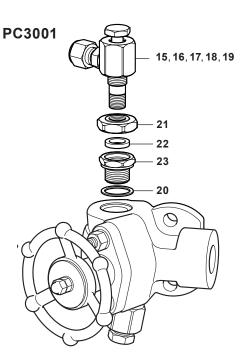
**Please note** The PC3001 and PC3000 unit is supplied fully assembled; the view is only exploded for ease of part identification.
