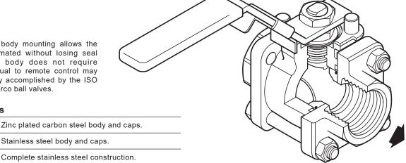
M10HTi3 ISO Stainless steel body and caps. M10HTi4 ISO Complete stainless steel construction.
