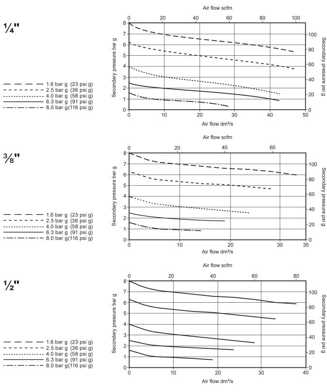
The graph utilises some typical values for secondary flow/pressure to demonstrate droop
