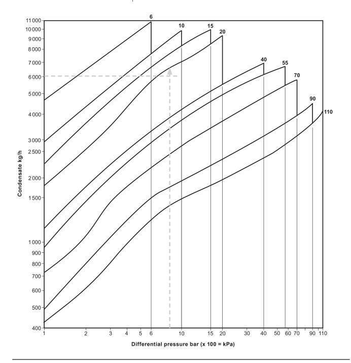
Note: IBV inverted bucket steam traps should be selected for use at the most appropriate working differential pressure and not on the basis of load.
