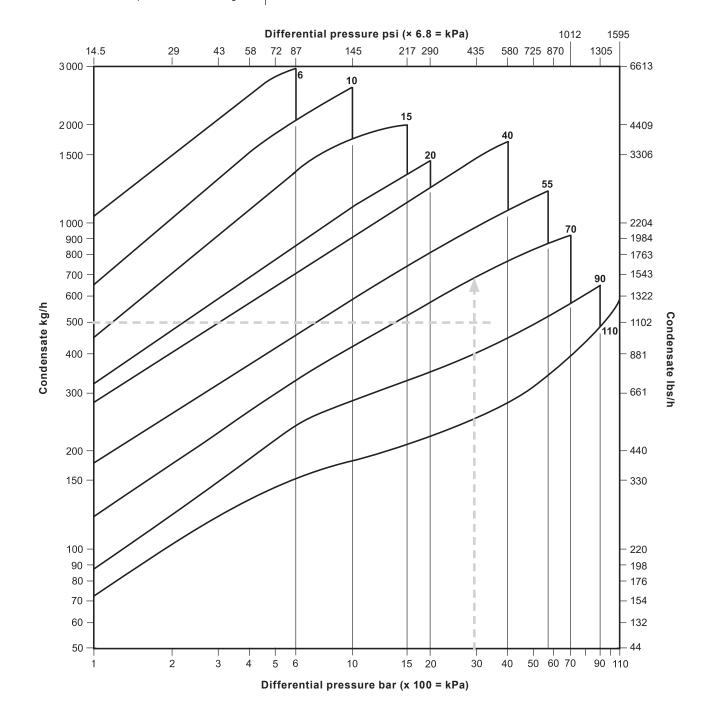
Note: IBV inverted bucket steam traps should be selected for use at the most appropriate working differential pressure and not on the basis of load.
