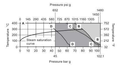
A-B-B Flanged Class 600, Screwed BSP/NPT, Socket weld and butt weld ends
