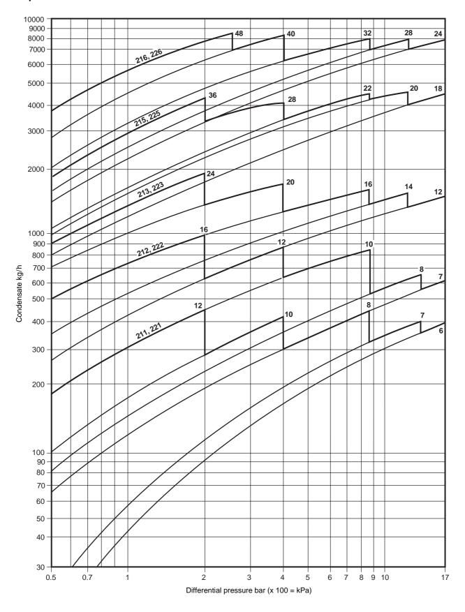
**Note**: Traps should be selected for the most appropriate working pressure differential and not on the basis of load.
