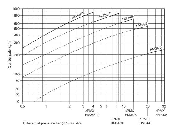
**Selection note:** Traps should be selected for the most appropriate working pressure differential and not on the basis of load, For example; DN25 HM34 with a load of 80 kg/h at 7 bar differential should be handled by an HM34/10 and not an HM34/5.
