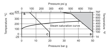
The product **must not** be used in this region or beyond the parameter of the PMA or TMA of the relative end connection.
