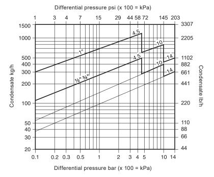
**Note**. Capacities shown are based on discharge at saturation temperature. When discharging sub-cooled condensate the air vent provides extra capacity. Under start-up conditions the thermostatic air vent will be open, and will provide additional condensate capacity to the main valve assembly. On 4.5 bar units this will provide a minimum of 50% increased capacity above the hot condensate figures shown.
