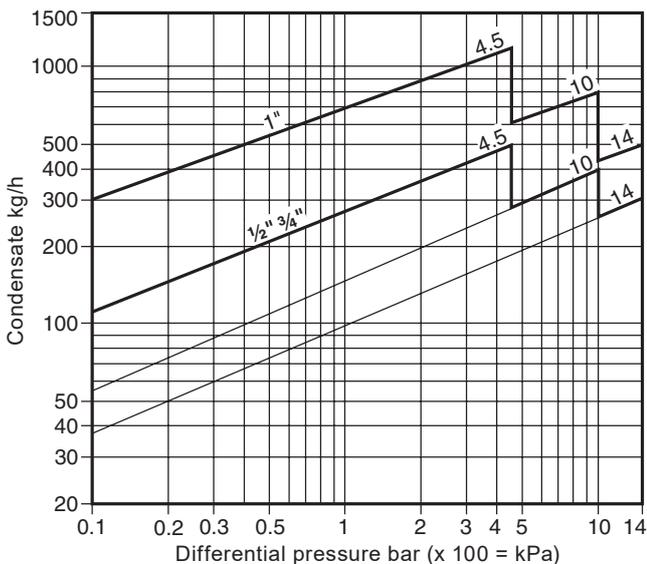
**Note.** Capacities shown are based on discharge at saturation temperature. When discharging sub-cooled condensate the air vent provides extra capacity. Under start-up conditions the thermostatic air vent will be open, and will provide additional condensate capacity to the main valve assembly. On 4.5 bar units this will provide a minimum of 50% increased capacity above the hot condensate figures shown. On 10 and 14 bar units this will be a minimum increase of 100% on the published capacity.
