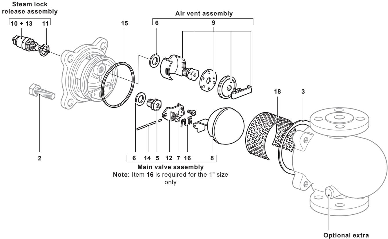
At extra cost the cover can be tapped 1/8" BSP T Rp (ISO 7-1) for installation of a temperature sensor.
