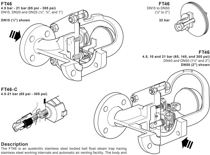
The FT46 is an austenitic stainless steel bodied ball float steam trap having stainless steel working internals and automatic air venting facility. The body and cover castings are produced by a TÜV approved foundry. The trap is supplied with integrally flanged connections and can be maintained without disturbing the pipework. Flow direction for the horizontal trap is clearly illustrated above.
