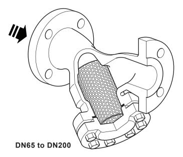
**Sizes and pipe connections**DN15, DN20, DN25, DN32, DN40, DN50, DN65, DN80, DN100, DN125, DN150 and DN200 Standard available flanges: EN 1092 PN16, AS 2129 table F
