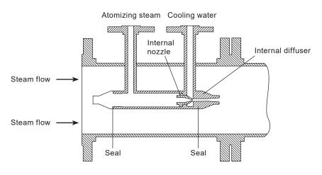
Finer droplets, therefore smaller absorbtion length and/or better turndown and approach to saturation
