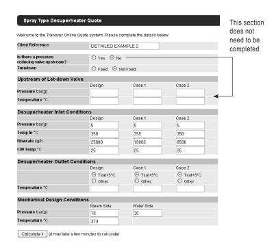
**Detailed example 2 (continued)** A Spirax Sarco Size 10 spray type desuperheater has been selected. The maximum cooling water pressure required is 140 psi g (9.65 bar g) and there is a negligible steam-side pressure drop.
