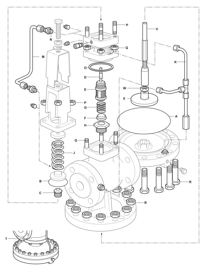
arrangement of main diaphragm chamber DN80 size only.
