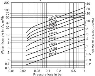
Pressure loss diagram with open valve at 20 °C. The values indicated are applicable to spring loaded valves with horizontal flow. With vertical flow, insignificant deviations occur only within the range of partial opening.
