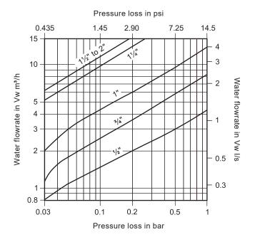
Pressure loss diagram with open valve at 20 °C (68 °F). The values indicated are applicable to spring loaded valves with horizontal flow. With vertical flow, insignificant deviations occur only within the range of partial opening.
