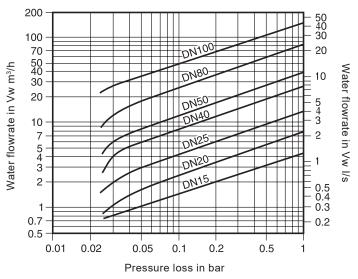
Pressure loss diagram with open valve at 20 °C. The values indicated are applicable to spring loaded valves with horizontal flow. With vertical flow, insignificant deviations occur only within the range of partial opening. The curves given in the chart are valid for water at 20 °C. To determine the pressure for other fluids the equivalent water volume flowrate must be calculated and used in the graph.
