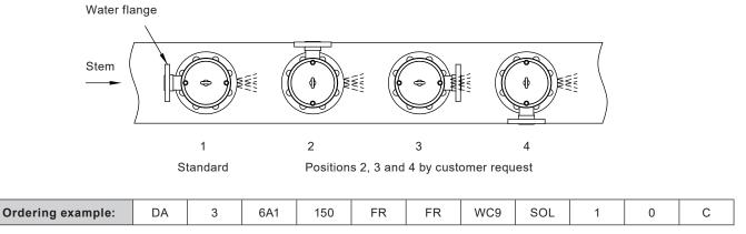
Desuperheater DA 3 inch nominal diameter with a Cv = 0.30, Steam and water ASME 150, flanged connections, body material ASME SA-217 Gr. WC9, integral flange, standard trim material, pneumatic spring return actuator with standard spring range.
