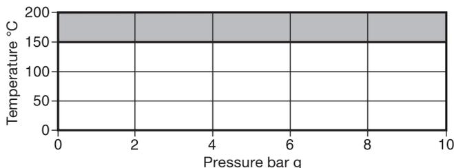
The CVS10 with EPDM seats **must not** be used in this region.
