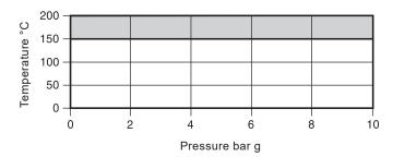
The CVS10 with EPDM seats **must not** be used in this region.
