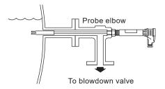
Typical horizontal installation on a boiler standpipe (screwed or flanged).
