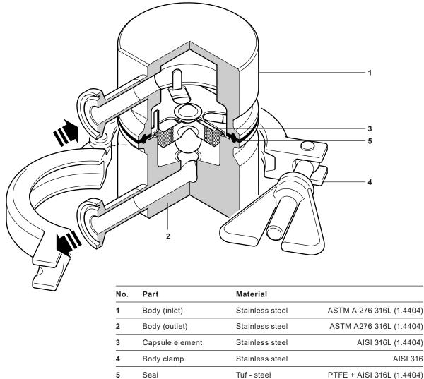
BT6B Horizontal Sanitary Balanced Pressure Thermostatic Steam Trap
