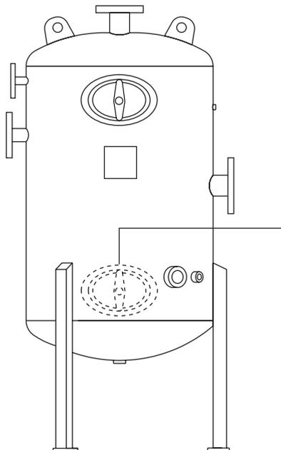
**Note:** There is a second inspection opening on the BDV60/6, BDV60/8 and BDV60/10 which is fitted 180° to the top opening. Other sizes have a single central opening, similar to the one shown on page 2.
