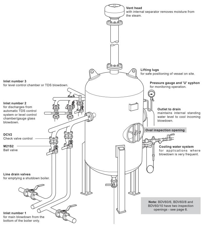
Vessel drain valve for clearing sludge from the blowdown vessel.
