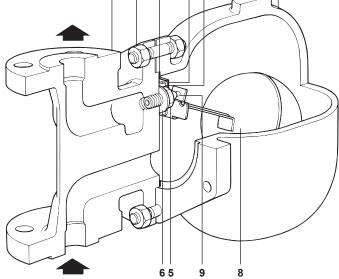
**Description and available types**The AE44 and AE44S are float type automatic air and gas vents for liquid systems. The body and cover are of steel and the valve cone is available in synthetic rubber designated AE44 or in stainless steel designated AE44S. Body and cover castings are produced by a TÜN approved founder. TÜV approved foundry.
